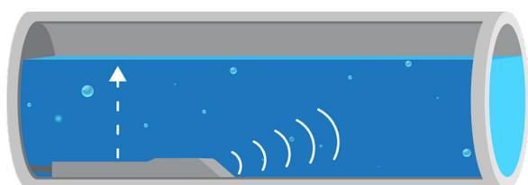
Submerged ultrasonic sensor measures level and velocity
